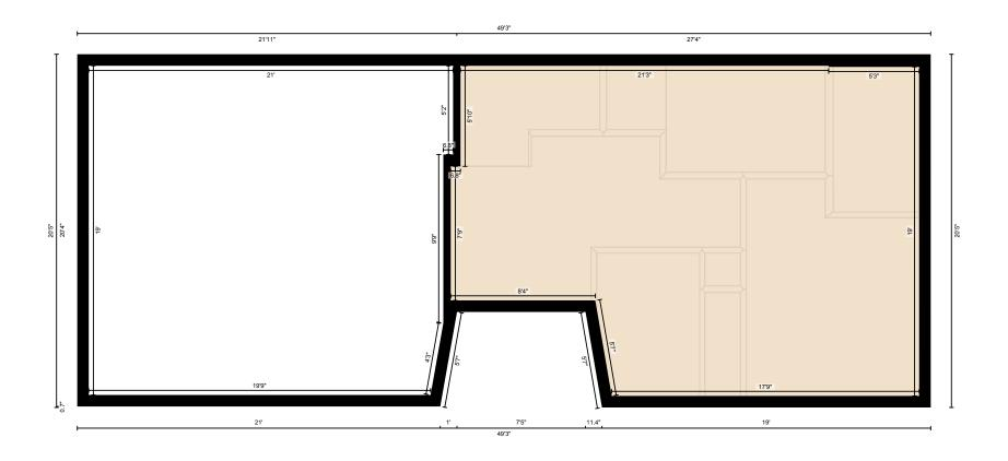
Measurement Diagram for: Main Floor Exterior Wall Thickness: 8.0 in
