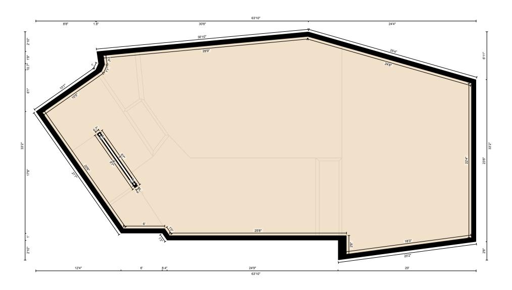
Measurement Diagram for: Upper Floor Exterior Wall Thickness: 8.5 in
