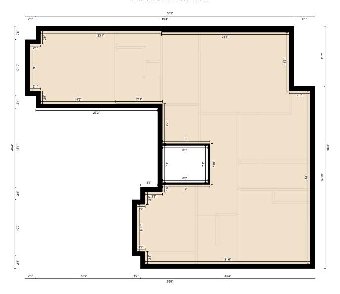
Measurement Diagram for: Lower Level Exterior Wall Thickness: 11.0 in
