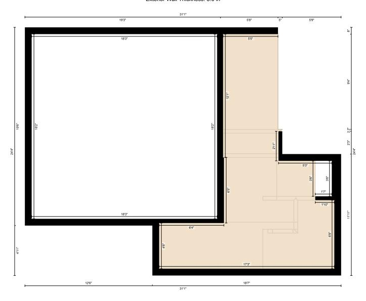
Measurement Diagram for: Lower Level Exterior Wall Thickness: 8.0 in
