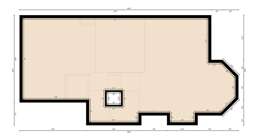
Measurement Diagram for: Upper Floor Exterior Wall Thickness: 8.0 in
