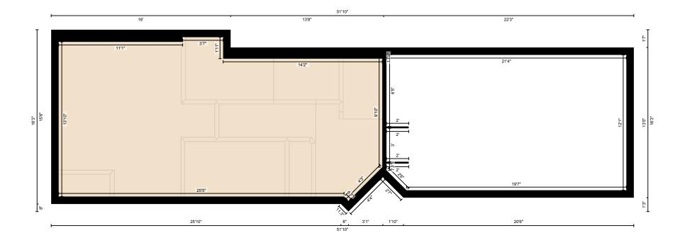
Measurement Diagram for: Main Floor Exterior Wall Thickness: 8.0 in
