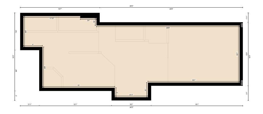
Measurement Diagram for: Upper Floor Exterior Wall Thickness: 8.0 in
