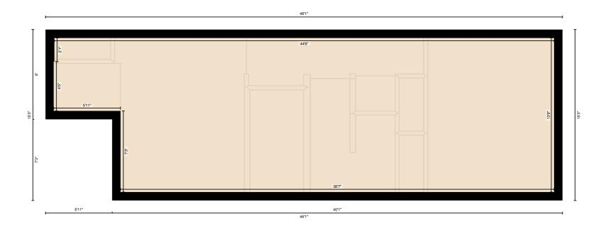
Measurement Diagram for: Lower Level Exterior Wall Thickness: 9.0 in
